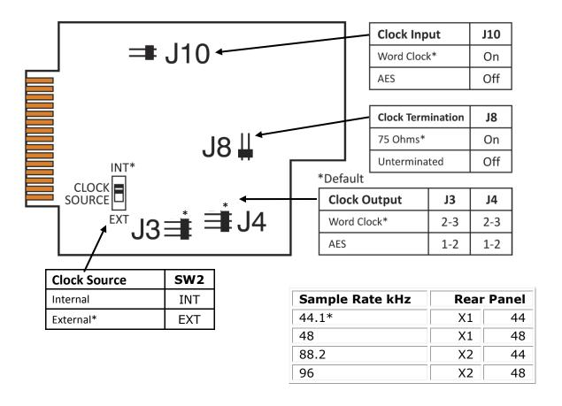
**Access Jumpers** by removing the cover from the HV-3D. The digita; I board has a diagram label showing the jumper setting and locations similar to the diagram on here.
