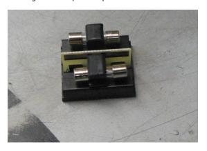
5. Make sure the voltage you want is showing in the little window and the arrow on the cover lines up with the arrow on the IEC power module. Press it back into the IEC power module.
