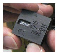
4. This is what the module looks like. The fuses used for 120V operation may be used for 240V operation.
