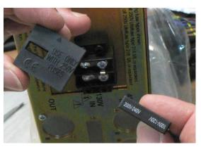
3. Turn the little card around so the voltage you want will appear in the little window and slide it back in. Notice the arrow showing the top of the fuse module.
